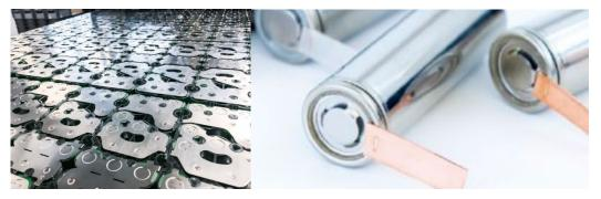
**Image 2:** Cost-efficient mass production only via automation: welded copper conductors with nickel coating on lithium-ion battery packs.
