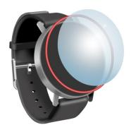
**Image 1:** Touch displays on smartwatch housings are sealed water-tight. The red adhesive element is fed fully automatically and is laser-activated.
