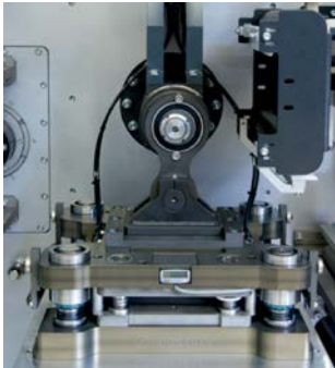
Image 1: Part of the Standard Production-Line for laminated Li-Ion Pouch-Cells: With the Highspeed Notching Platform Manz offers a highly efficient solution for the manufacture of individual electrodes or electrode webs.
