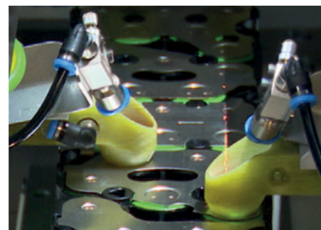
Tab welding on battery cells
