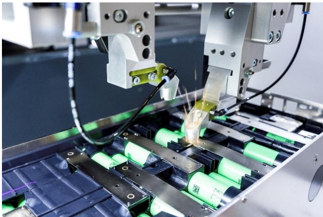
Caption: Laser Tab Welding process with BLS 500
