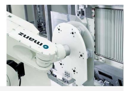
The first industrial jig free vertical plating production lines improve product yields and maintain optimal conditions for further processes after plating.
