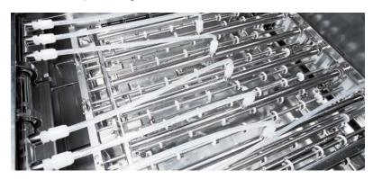
100 % photoresist removal and no remaining photoresist on the substrate after stripping processes
