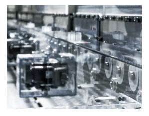
Providing outstanding etching stability and uniformity, the systems remove partial metal thin film layers to form excellent circuit patterns with acid chemicals.
